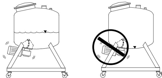
Dry operation of the Sanimixer 3000® will damage the bearing.
