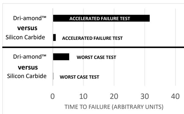
■ **Figure 1** Steridose Dri-amond™ bearings time-to-failure under adverse running conditions versus standard silicon carbide. Refer to the text for descriptions of 'worst case' and 'accelerated failure test'.
