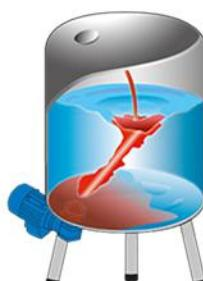
2- After reaching the impeller, the fluid flows in a radial direction towards the vessel wall.
