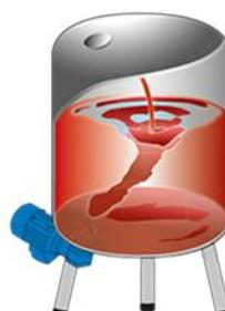
3- After reaching the vessel wall, the fluid travels upwards and then circulates down to the impeller again. The overall bulk movement and the mixing action around the agitator ensure that a homogeneous concentration distribution is achieved.
