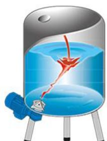
1- Soluble powder or liquid is added into the vortex. It is then rapidly transported downwards to the impeller.
