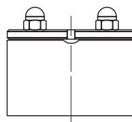
Sterisample fits in the following clamp connection Steriflange ASTM M-100 (metric), and ASTM I-100 (inch), and can be supplied in the following four sizes, 12, 25, 38, and 51 mm.
