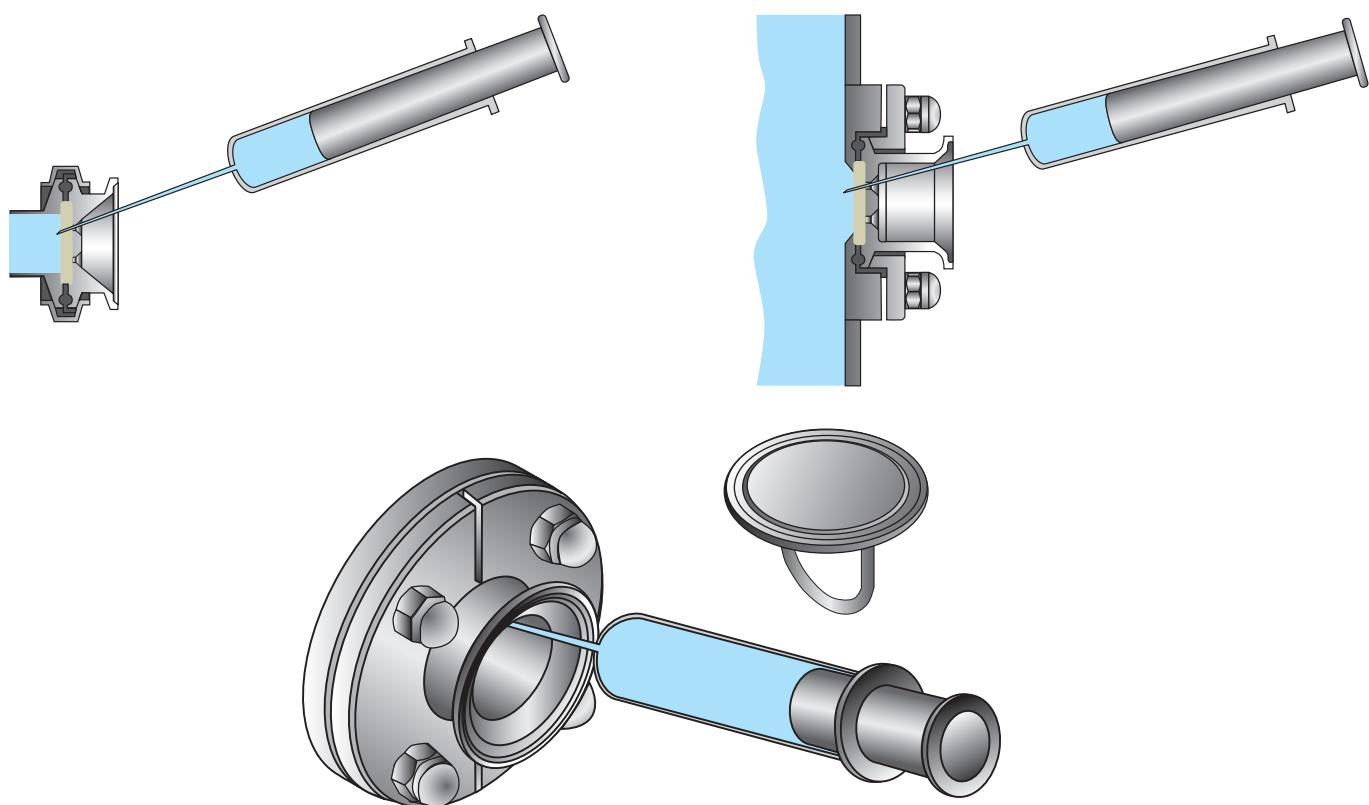
Sterisample short, for standard TC-flange Connection
